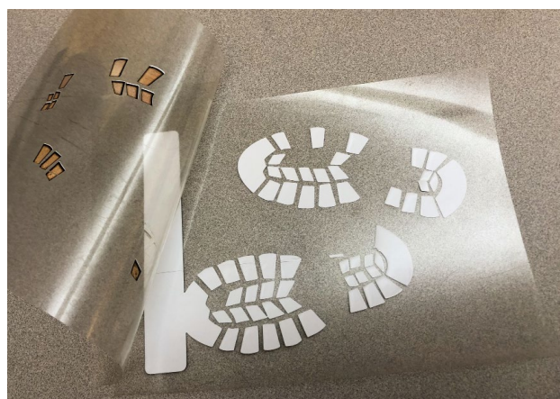
FIG 2: The printed graphic is not completely transferring to the heat transfer tape. A higher-tack tape or more squeegee pressure is needed.
