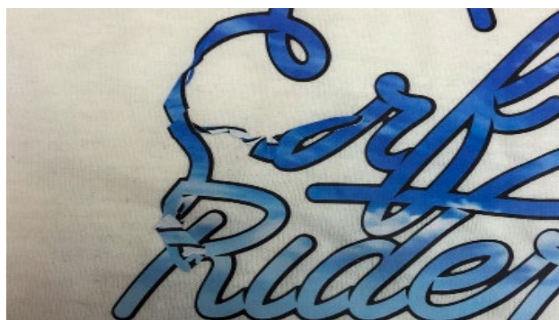
FIG 1: Using ClearMASK MT with WarmPEEL CP PRINT can cause this issue. CP PRINT requires a lower-tack transfer tape.
