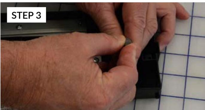
Push the new plug about half way into the tube connector. Then, while pressing the choke valve lever, push the plug in completely. Install the tube connector back to the ink adapter tabs securely.
