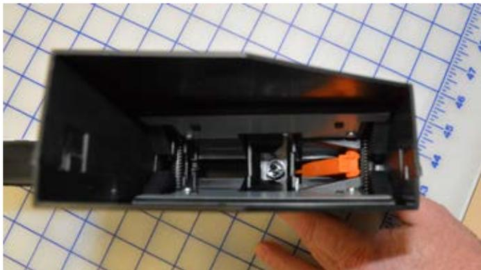
The top picture shows the orange Lock lever located on the lower rear of the adapter cartridge. Holding the orange tab down opens the inner channel to allow the ink bag to settle into the cartridge, as seen above.
