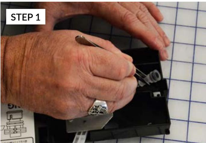
To replace the plug, remove the adapter from the printer and wipe off the excess ink. Then take a fine-tip tool, like tweezers or a precision screwdriver to push the tube connector out.
