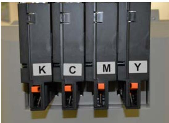
The high capacity ink adapter kit comes with a set of five labels: one each for Cyan, Magenta, Yellow, Black, and cleaning (CMYK Cln). After inserting all of the ink adapter cartridges, apply the correct ink label to each adapter, as seen at left, so that there will be no confusion in the future when new ink bags are installed.
