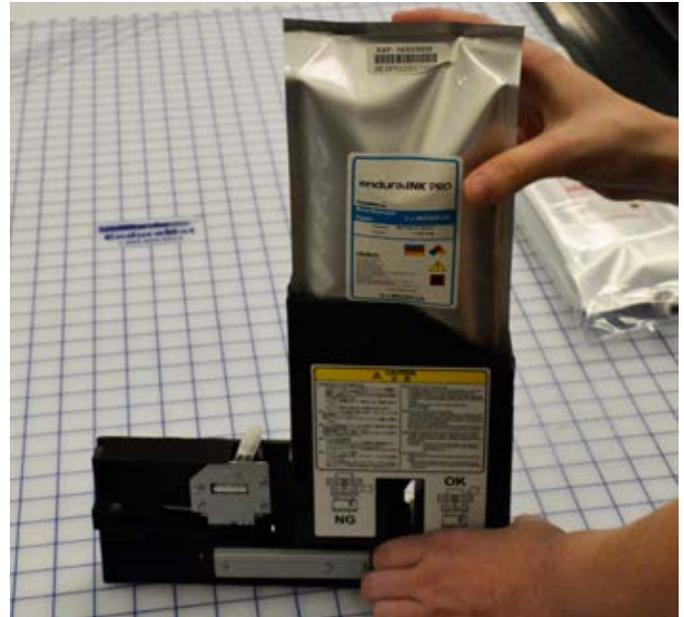
Lower the ink bag into place so that the nozzle of the ink delivery neck fits into the needle. To ensure a good seal, firmly tap the cartridge on a firm surface to make sure it's fully seated. While holding the lock tab down, gently push the bag until the rings on the nozzle are below the locking tab, as seen below.
