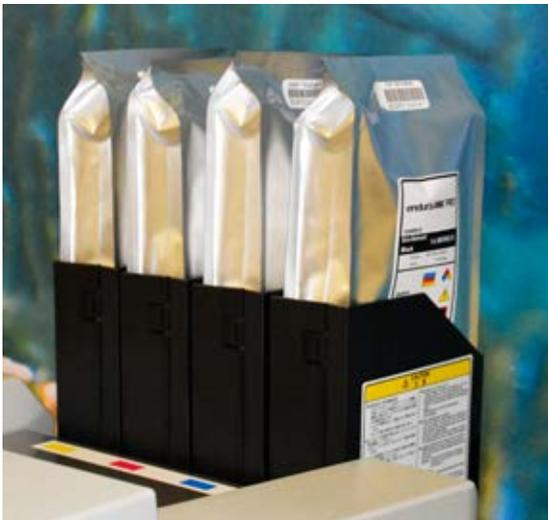
Remove the original 220ml ink cartridges one at a time, allowing time for the printer to register that the slot is empty with an alarm and a "No Cartridge" message on the control panel.
