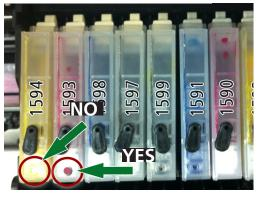
Remove the film that covers the breather hole at the back of the ink cartridge by pulling on the yellow tab. The film can sometimes tear, leaving the clear end over the hole. Be sure to remove it completely. The plastic breather hole must be completely uncovered or ink will not flow through the print head.
