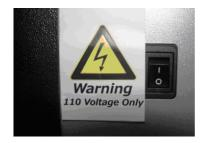
Remove the label over the electrical input module. Compare the voltage on the label to the voltage of the location where the printer is being installed. If they match, plug the power cord into the back of the printer and flip the power switch to On.
