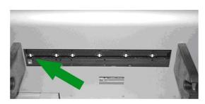
Feed the end of the media into the roll feeder. The media should go directly under the little white rollers you see in the slot.
