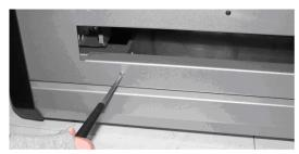
Remove the screws and keep them. These will be used for the media output tray installation.
