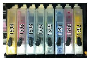
Open the carriage cover and install the ink cartridges.
