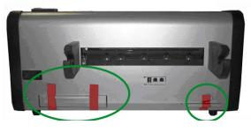
Remove the tape from the waste ink drawers located on the back of the printer on the left and right side.
