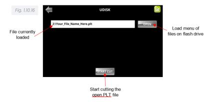
Press **START CUT** to cut the .PLT file. Note that if you want to cut repeats refer to the Array function covered in *Section 10.8.4*.
