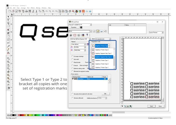
4.7 If you are producing a large number of copies, you can opt for the Segmented registration marks option. This optionadds sets of registration marks that divide the batch of decals into segments that are scanned and contour-cut in sequence. This enhances the accuracy of the contour-cutting and is recommended for cutting jobs over 4 feet in length. To activate this, choose Graphtec Segment Area Type 1 or Graphtec Segment Area Type 2 from the registration marks drop-down menu.
