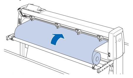
4 Lock the media stopper (Raise while pulling forward) and pull it out evenly so that the roll paper is straight. Please load so that the roll paper always rests on the media sensor.
