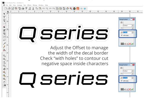
Use the Offset window to determine the width of the border between the edge of the printed area and the intended cut path. For a full-bleed decal, select a negative value in the offset window. Be sure to click the green check mark or press the Enter key to apply the settings previewed in Design Central.
