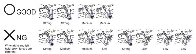
When using three push rollers
