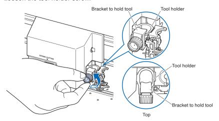
While pushing up the tool holder, push until its flange completely touches the upper part of the holder.
