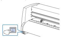
Connect one end of the provided power cord to the Q Series Cutter AC line inlet and the other end to an electrical socket of the rated supply voltage.
