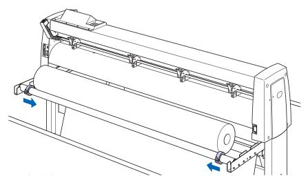
Push the tip of the roll media forward from the back of the Q Series Cutter. Make sure to pull it so that there is no slackening across the roll media's route.
