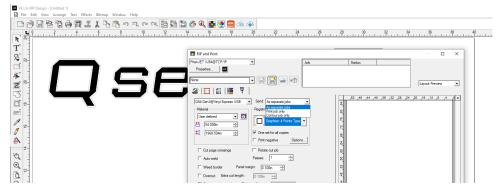
**4.4:** LXi loads cutter drivers with default settings that override the speed, force, and offset values on the cutter. You will see these in the Driver Options window at the bottom of the Contour tab. Click Edit and, from the Vinyl Express driver options pop-up window, click the Cut Fast default. From the drop-down menu, select None, then click the Apply button in the lower right corner.
