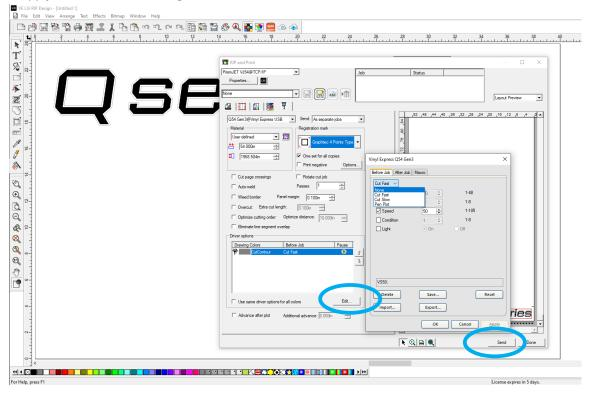
4.5 If you wish to print and cut multiple copies of a design, use the Copies function in the General tab to determine the number. Use the horizontal spacing and vertical spacing windows to manage margins between the rows and columns. The default setting expands the registration marks to form one bracket around the pattern of decals. This will create one set of marks that the Q Series cutter will scan before contour cutting.
