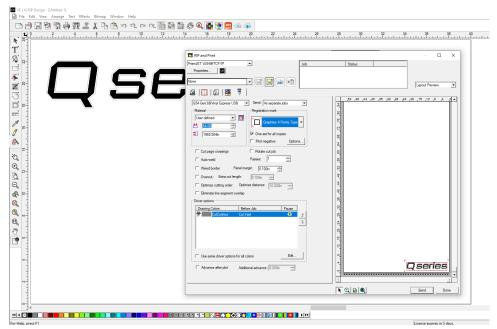
4.3 Click the Send window on the Contour tab and, from the drop-down menu, select, "As separate jobs." This will send the raster data to the printer and send the vector data to the cutter. The vector data will be held in the Production Manager queue for the Q Series cutter.
