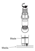
2 Extend the blade little by little to the thickness of the media. Optimal blade length is less than the thickness of film and backing sheet combined, but more than the thickness of the film.
