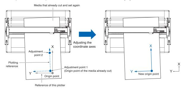
There is a misalignment between the X-Y axis and origin point of the plotter and the media plotted.
