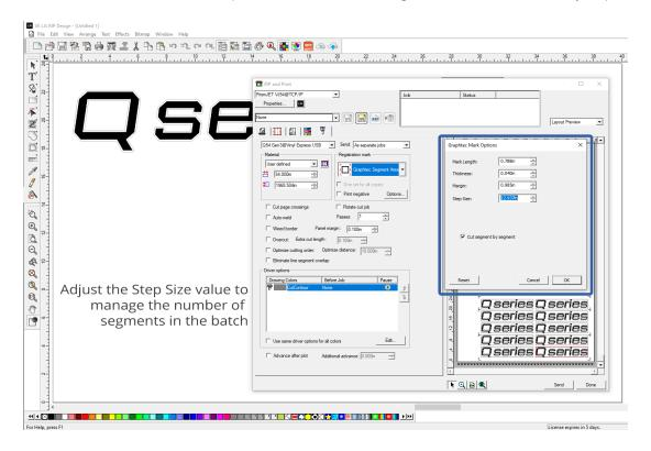
4.9 You can also use the General Tab's preview window to adjust the margins between the rows to align the segment marks with gaps between batches of decals. Use the Vertical Spacing setting in the Copies window to make this adjustment.
