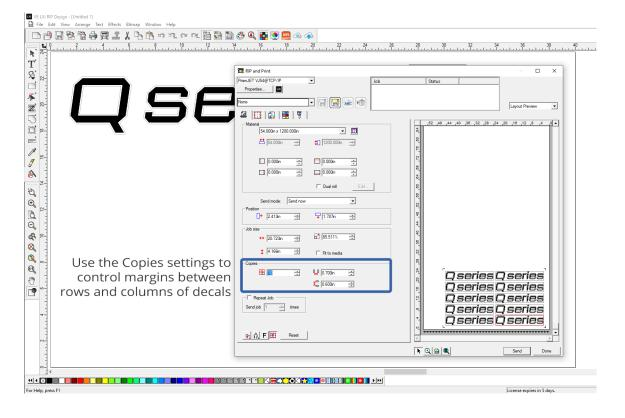
4.6 As noted in section 13.1.3, select Graphtec 4-point Type 1 or Type 2 to add one set of brackets around the marks. Make sure "One set for all copies" is checked.
