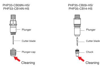
2 After completing cleaning, attach the plunger cap or the chuck.
