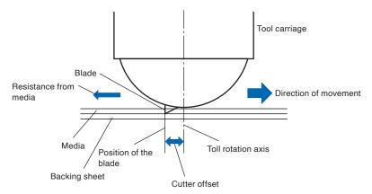
The blade tip gets stuck in the media with 0.3 mm or thicker, making the blade hard to rotate. Especially for the corners where two straight lines meet, cutting becomes very hard because it cannot rotate smoothly.
