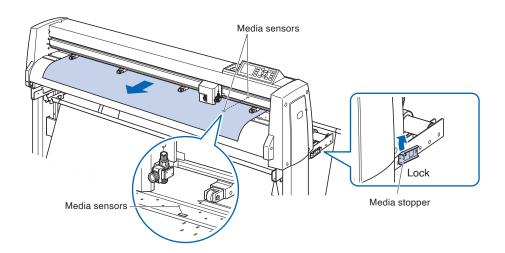
5 Position the media and the push rollers to correspond with the width of the media.
