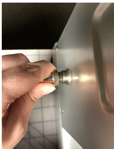
FIG 1: Disconnect the power cable before removing the fitting.
