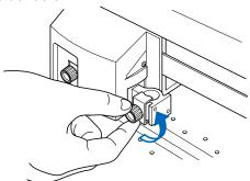
While pushing the pen holder in the upward direction, push the pen all the way into the holder until its flange contacts the upper part of the holder.
