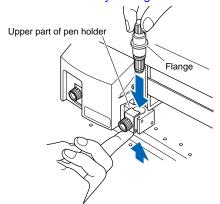
3 Make sure that the pen bracket is engaged on the pen's flange, and then tighten the screw.
