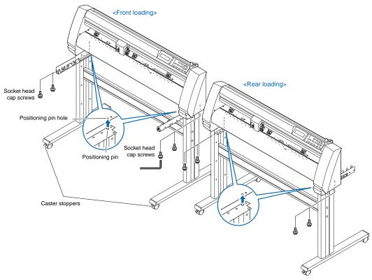
5 Tighten the socket head cap screws loosely fastened in Step 2.
