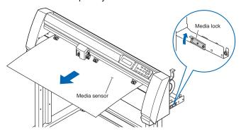
4 Pull the media taut to make sure that there is no slack in the conveyance path, and then raise the media set lever to lower the pinch rollers. Release the media lock.
