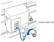
3 Remove the protective cover from the replacement cross-cutter unit. Be sure to remove the protective cover while holding the part of the unit shown in the figure below.
