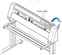
2 Place the media roll on the roll media stocker. Load the media in the plotter as shown. Pass the leading edge from the front of the plotter so it emerges from the back.
