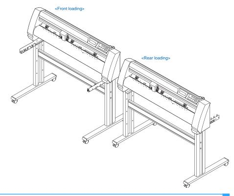
1 Assemble the left and right stand sides. Fasten a base assembly to each of the stand side bars with four socket head cap screws, using the Allen wrench.
