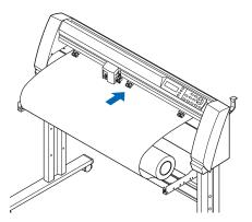
3 Press the media lock to engage it, and then pull the leading edge out of the back of the plotter so that it completely covers the media sensor.
