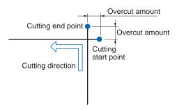
1 Press the function key **F1** through **F4** corresponding to the cutter-pen setting area for which tangential emulation is enabled, and which requires an overcut setting. Number 4 is used for the explanations in this section.
