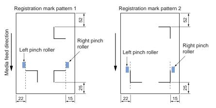
With roll media, the registration marks must be at least 110 mm from the back edge of the media.
