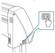
2 Connect one end of the provided power cord to the Vinyl Express AC line inlet and the other end to an electrical socket of the rated supply voltage. Make sure that the Vinyl Express is grounded.
