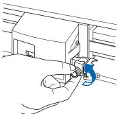
While pushing the pen holder in the upward direction, push the pen all the way into the holder until its flange contacts the upper part of the holder.
