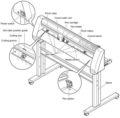
Pen carriage: ......Moves the cutter-pen or plotting pen across the media during cutting or plotting.
