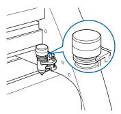
3 Close the pen-hold mechanism on the pen station to hold the pen in place.
