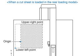
When ROTATE has been selected to rotate the coordinate axes by 90° as shown in the example below, the shaded area represents the effective cutting/ plotting area defined by the LL and UR points.
