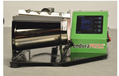
FIG 3: Some fittings are conical and designed for tapered drinkware.
